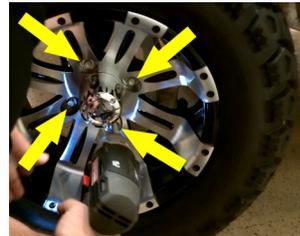
**NOTE:** It is recommended to use at least 22" tires on a 10" wheel with an offset. The wheel shown is a *RHOX Vegas TIR-RX160* with a *RHOX Mojave* tire, TIR-265.
