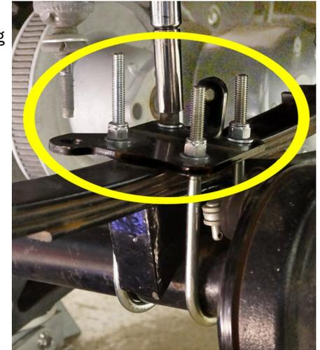
10. Fully tighten both U-Bolts. Adjustments may be needed to maintain alignment.
